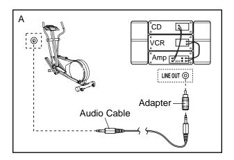
B. Plug one end of the audio cable into the jack beneath the console of the elliptical crosstrainer. Plug the other end of the cable into the included adapter. Plug the adapter into an RCA Y-adapter (available at electronics stores). Next, remove the wire that is currently plugged into the LINE OUT jack on your stereo and plug the wire into the unused side of the RCA Y-adapter. Plug the RCA Y-adapter into the LINE OUT jack on your stereo.
